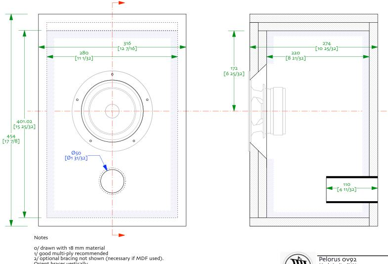
Orient braces vertically 3/ line all internal faces with damping 15mm - 20mm [3/4in] wool felt or similar [blue on drawing]. Avoid foam. 4/ If 2in vent used it dhould be 4.375in 5/ open up back-side of driver cutout (45° bevel shown)
