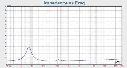
FS 77.7903 Hz VAS 4.4905 L RE 3.5000 Ohm QMS 2.7968 QES 0.6623 QTS 0.5355 Bxl 2.9146 dBSPL87.063 SD 0.0050 m2 CMS 1.2728 mm/N MMS 3.2888 g MMD 3.0871 g L1kHz0.0274 mH PWR 15 Watts Nom X max (Mech) +/- 4mm
