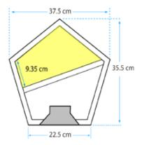
The line is open at the top (shown in yellow on plan view). Vertical braces can be fitted to bridge the sides and partition; these can be small panels of 18 mm ply (shown in blue) or dowels. These also help support the stuffing material.
