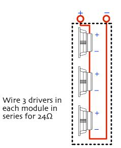
Wire modules in parallel [3 modules =  $8\Omega$ ], [4 modules =  $6\Omega$ ], [5 modules =  $4.8\Omega$ ], [6 modules =  $4\Omega$ ]
