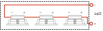
All drivers wired in series, as in a mains module, for an impedance of  $24\Omega$ , Most modern HT receivers will have sufficient power despite a reduction in power to 1/3 the rated power into  $8\Omega$ . Note that distortion will also decrease.
