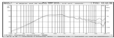
Illustration of a measured array response, un-equalized on axis and 30 degrees off axis
