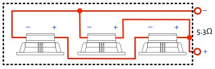
**Recommended:** Outer drivers wired in series, these wired in parallel with the centre driver for an impedance of  $5.3\Omega$ . This will create a tapered array with the centre driver having 3dB greater output than the end drivers.
