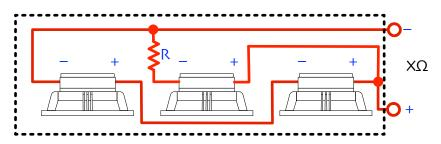
This is a variation of the scheme above (above R=o). With R=8 $\Omega$  there is no power tapering and the outer drivers will have the same output as the centre driver (net impedance of the module is 8 $\Omega$ ). The resistor will need to be able to handle 1/4 the power input. Decreasing the resistor value from 8 $\Omega$  will increase the power tapering until maximum is reached when R=o (as above)
