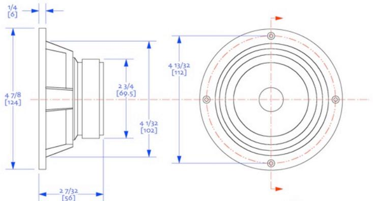
Note that these come with a 2mm gasket, which doesn't compress very much, so it needs to be accounted for when cutting the rebates.
